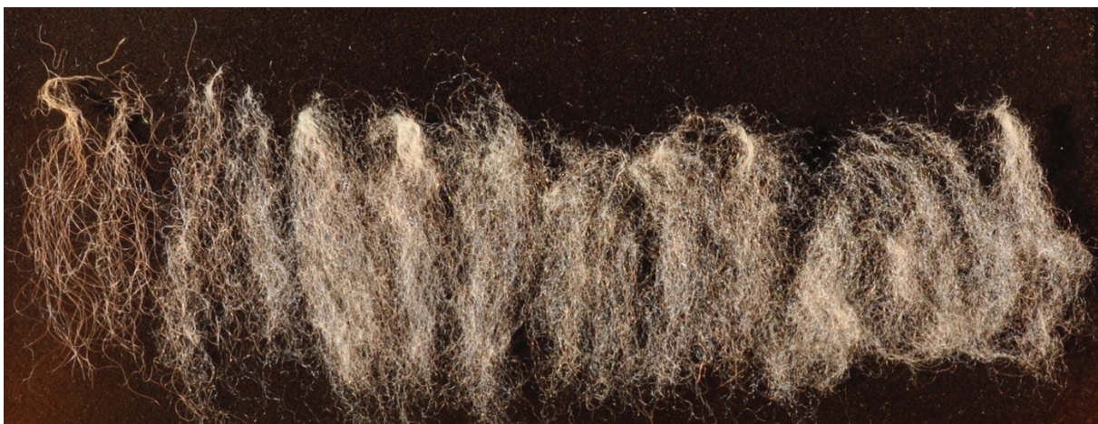
Figure 1: DC staple fibres placed on a velvet cloth in accordance with Baer Diagram (Onions, 1962).
